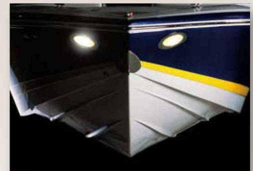
Deep-V Hull and Reverse Chines
